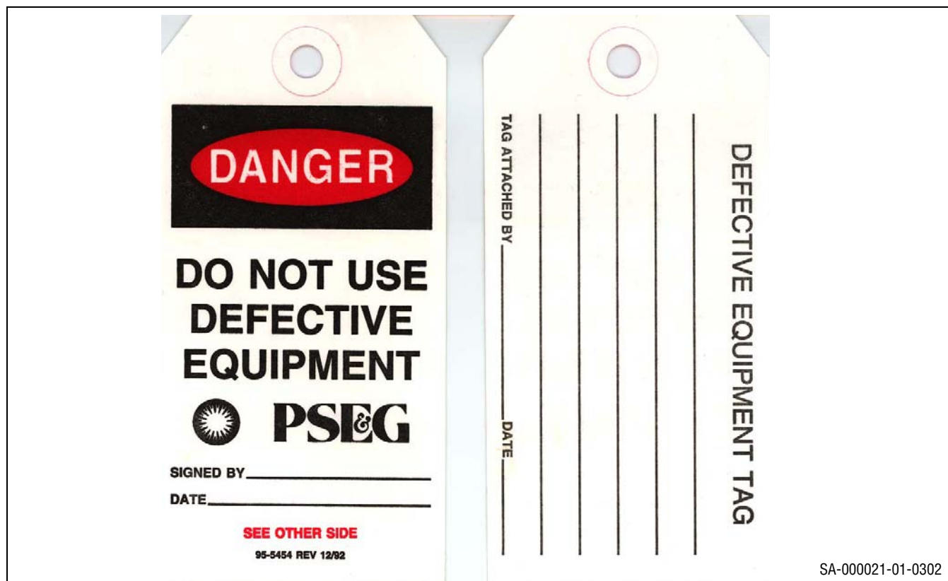
Figure 7.1: Defective Equipment Tag (PSE&G Form 95-5454)
