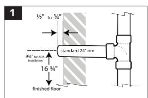
**SET DRAIN LINE HEIGHT** 16 ¾" from finished floor (standard 24" rim) or 9¾" for ADA installation. Threaded nipple should extend ½ to ¾" from wall.
