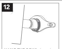
HANG THE BOWL, inserting tailpipe into bushing, then install anchor screws with washers. TIGHTEN FLANGE BOLTS AND GEAR CLAMP.
