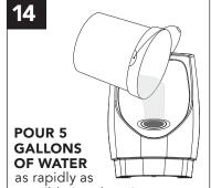
as rapidly as possible into housing to ensure good flow and no leaks or standing water.
