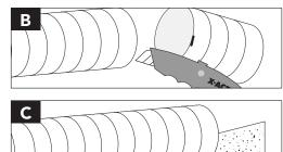
**B. Cut the tube** at the groove using a sharp utility knife to ensure a square, flat cut. **C. Clean burrs** from the cut end by using
