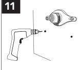
**DRILL HOLES** with 5/16" masonry bit for the lower anchor screws and insert plastic anchors.
