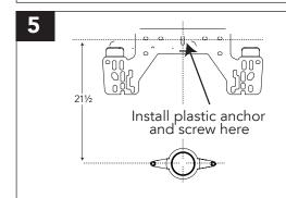
**MEASURE & MARK THE ROUGH-IN** is in-wall carrier is not used. Use a 5/16" masonry bit to drill hole, then install the hanger bracket with one plastic anchor and screw.
