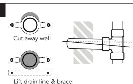
Lift drain line & brace with mending plate
