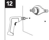
**DRILL HOLES** with 5/16" masonry bit for the lower anchor screws and insert plastic anchors.
