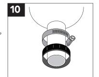
PLACE THE GEAR CLAMP and compression nut onto the housing tailpipe.
