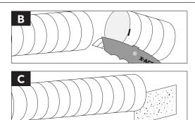
B. Cut the tube at the groove using a sharp utility knife to ensure a square, flat cut.
