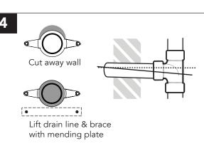
**ADJUST DRAIN TO ACHIEVE PITCH** only if standing water is present (code requires ¼ "drop per foot of drain line for proper pitch). Seal wall according to code.
