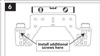
**LEVEL THE BRACKET THEN MARK,** drill and install two additional plastic anchors and screws. If pre-existing bearing rods can be used, screws are not necessary.
