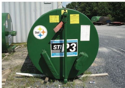
Figure 3-12: Underground steel tank
