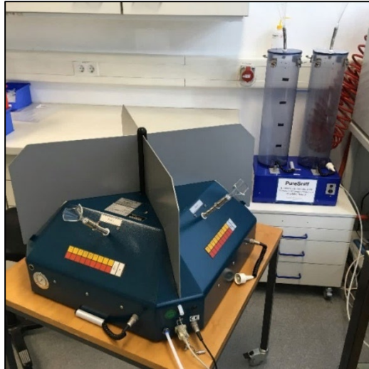
Figure 5: Olfactometer (left) and odor presentation device for air sampling bags with gas connections (right). Printed with permission of BMW Group.
