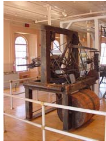
The Blanchard stock-making replicating lathe, built 1822, seen at Springfield Armory NHS
