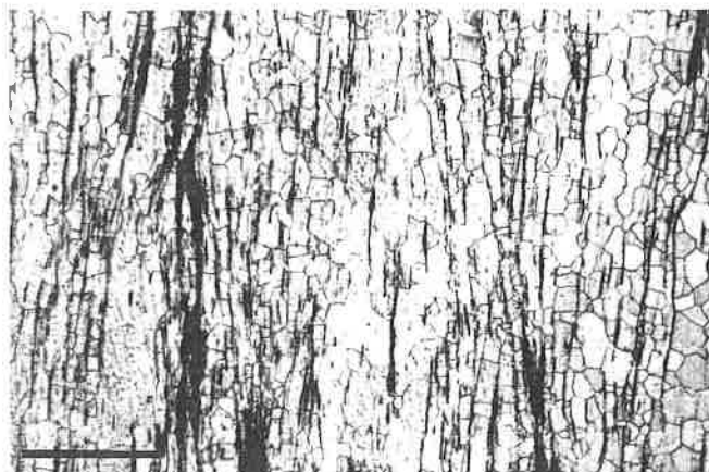
Figure 3: The slag fibres in the shank of nail 8 are oriented parallel with the length of the shank (vertical in the image), thereby showing the longitudinal orientation of a nail. Nital etch; length of scale bar 0.2mm.
