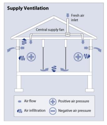
Supply ventilation systems allow better control of the air that enters the house than do exhaust ventilation systems. By pressurizing the house, supply ventilation systems discourage the entry of pollutants from outside the living space and prevent backdrafting of combustion gases from fireplaces and appliances. Supply ventilation also allows outdoor air introduced into the house to be filtered to remove pollen and dust or dehumidified to provide humidity control.
