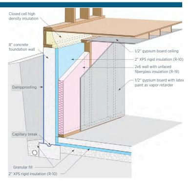
Basement walls can be insulated with rigid foam. For moisture control, the panels must adhere completely to the foundation wall, with no air gaps behind them, and edges and seams must be tightly sealed. Another option that avoids moisture problems is to use insulated concrete form foundation walls with a layer of foam inside the walls.
