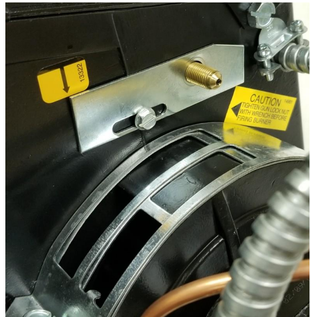
Figure 10 EH/EHASR Oil Gun Lock Nut Removal
