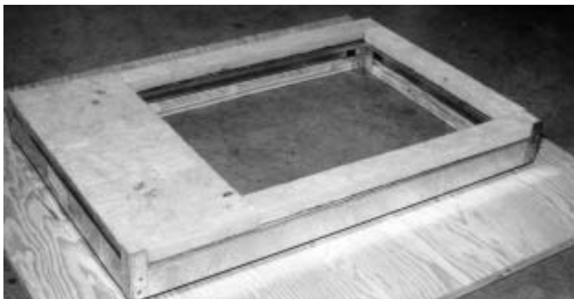
FIGURE 4 COMBUSTIBLE FLOOR BASE
