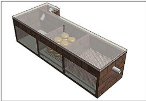
Figure 10. Gravel (3-6mm in diameter) filter materials in the Filter unit
