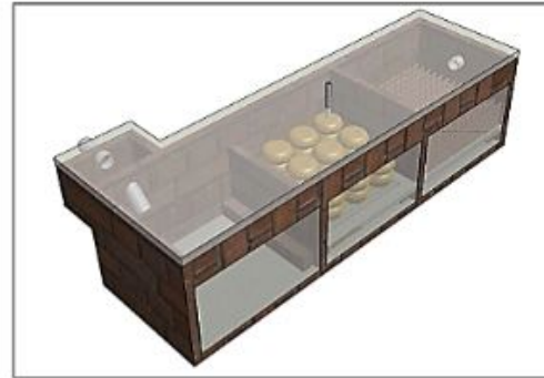
Figure 11. Gravel (3-6mm in diameter) filter materials in the Filter unit
