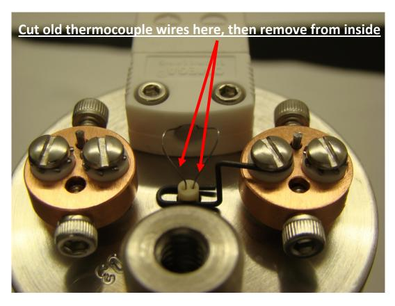
2. For Radak I and II models, remove the ceramic insulator post by removing the 4/40x7/16 screw that holds it to the power terminal. Then disconnect the spring by removing it from the notches in the ceramic post. For Radak III models, remove only the inner ceramic insulator which should be free to slide out once the thermocouple wires are removed.
