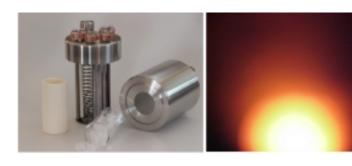
The thermocouple in your RADAK furnace has been made, installed, and inspected with great care. The junction, which is formed by spot-welding, is subject to failure due to mechanical or chemical stress. Vibration or some metal vapors, such as zinc, will occasionally cause failure in these thermocouple materials. If it is necessary to replace a thermocouple, please begin by taking a close look at the existing thermocouple leads. Then, we suggest the following:
