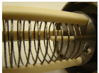
9. **For Radak III Furnaces:** Slide the new thermocouple leads into the inner ceramic post. Insert this ceramic post through the outer ceramic sleeve from the inside of the furnace.
