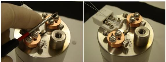
11. Loosen the terminal screws on the plug and wrap each wire around the appropriate screw about 3/4 of a full turn. Wrap from the inside of the plug to the outside. Tighten down the screws.
