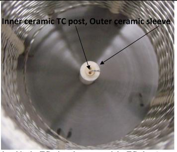
10. Put a small radius bend in the TC wires down toward the TC plug (a screwdriver shaft is useful for bending the wires).
