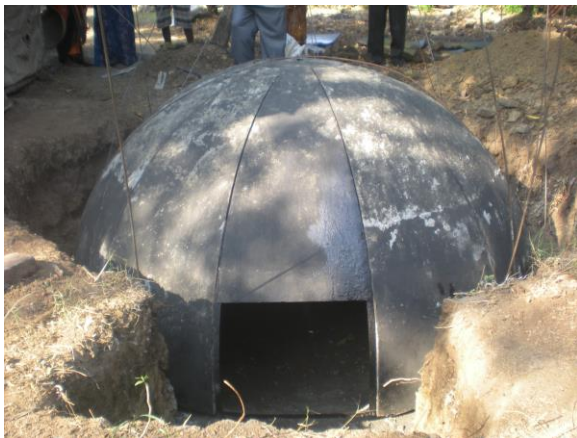
Fig. 4.19, A mild steel mold (Photo: PK Jha 2014)
