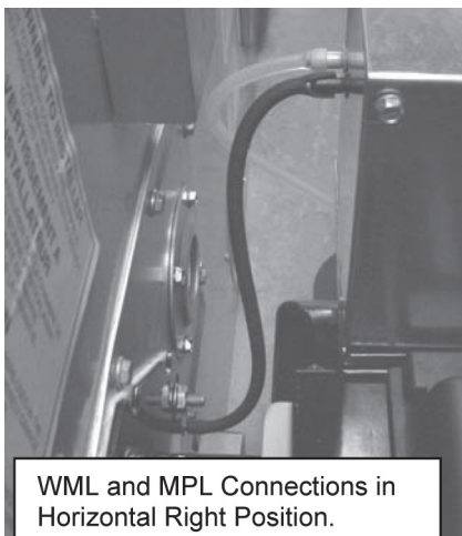
Figure 9 - Horizontal Right Connection
