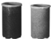
Fig. 8: Ruined cartridge filter
