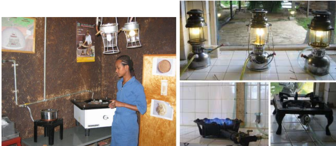
Figure 3.8 Utilization of biogas for gas stove and mantle lamp
