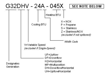
Note: Revision level will appear in the revision block below the model number on Nameplates. Bill of Material spreadsheets will show the revision level at the end of the model number.
