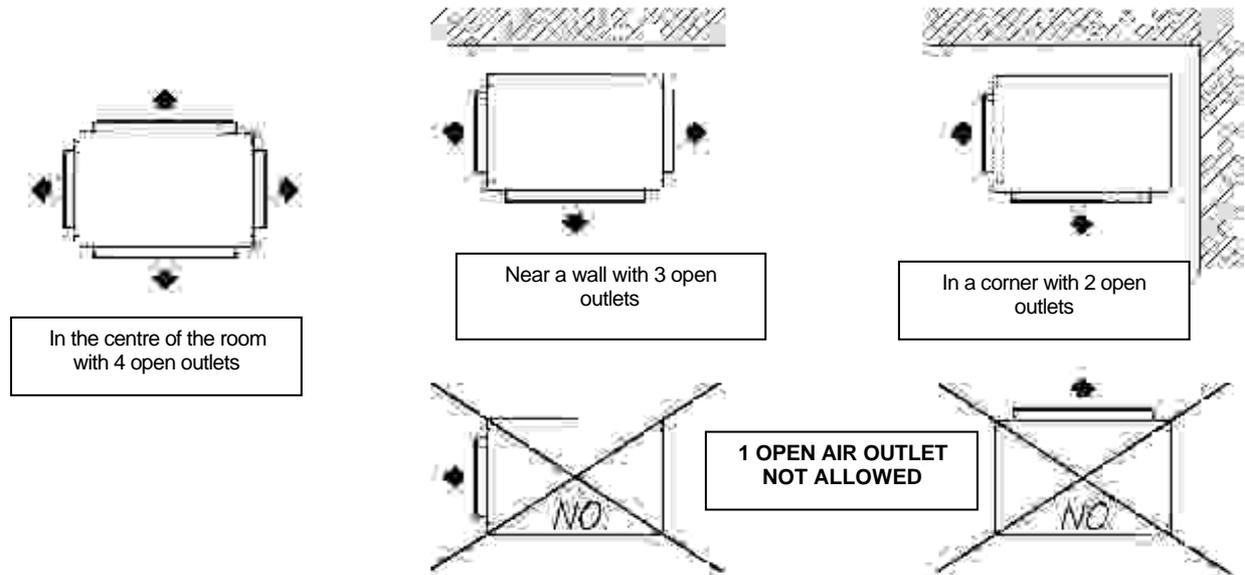
The heater is equipped with a 4 way head with movable flaps.
