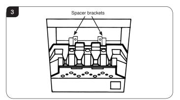
7.2 Locate the rear panel against the spacer brackets, see Diagram 3 and slide down so that it locates on the ledge of the flame baffle, see Diagram 4.
