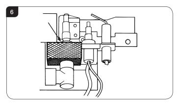
4.3 The pilot unit can now be removed by undoing the two screws, see Diagram 7.
