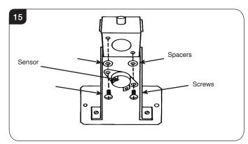
10.8 Feed the cable back through the hole as you replace the bracket.
