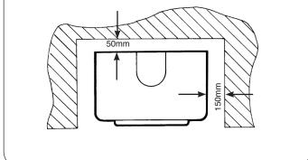
4.5 The above dimensions provide adequate clearance to combustible materials. It may be necessary to add additional clearance so that spillage tests can be performed when necessary.
