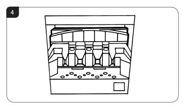
7.3 Locate the front coal between the heat shield and the flame baffle so that the ends sit flat against the burner skin, see Diagram 5.
