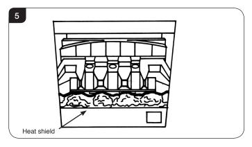
7.4 Place five of the loose round coals on the front coal so they lean against the flame baffle, in between the fingers. Place the two rectangular coals against the reflector panels, one either side, behind the front row of loose coals, see Diagram 6.
