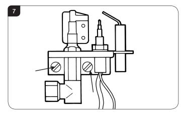
4.4 Reassemble in reverse order, do not overtighten. NOTE: SPECIAL CARE SHOULD BE TAKEN WHEN REPLACING THE THERMOCOUPLE TO THE BACK OF THE GAS VALVE TO ENSURE THAT THE SENSOR WIRES FOR THE GAZCO FLUE SURE SYSTEM ARE NOT DISCONNECTED.
