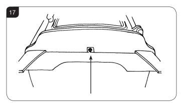
11.2 Undo the M5 nyloc nut from the bottom of the burner unit and remove the aeration plate, see Diagram 18.
