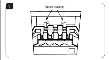
7.2 Locate the rear panel against the spacer brackets, see Diagram 4 and slide down so that it locates on the ledge of the flame baffle, see Diagram 4.
