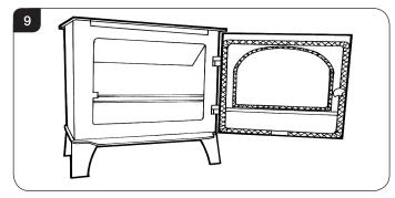
7.8 Secure door by tightening the grub screw with the 2mm Hexagon key.
