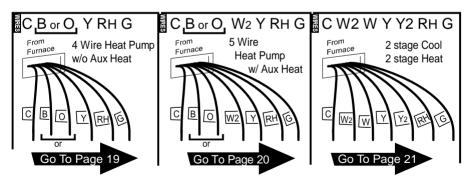
If your combination of wires is not above you can use the wiring table on pages 24-25 to determine your connections, or call our USA support line at 1-888-607-5824 for help.
