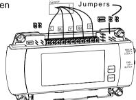
sure your wires are labeled. This may require you to find the 'other end' connection for each wire on your heating or air conditioning equipment and read the label there.
