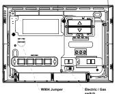
If you have either a gas or oil furnace, set the switch to GAS.
