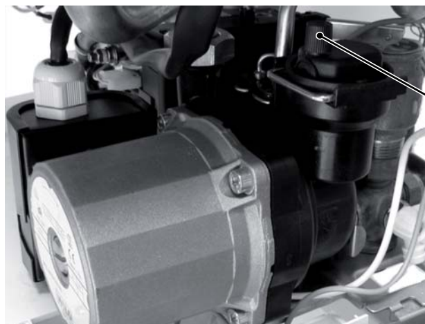
Figure 12.1: Location of Automatic Air Vent Cap
