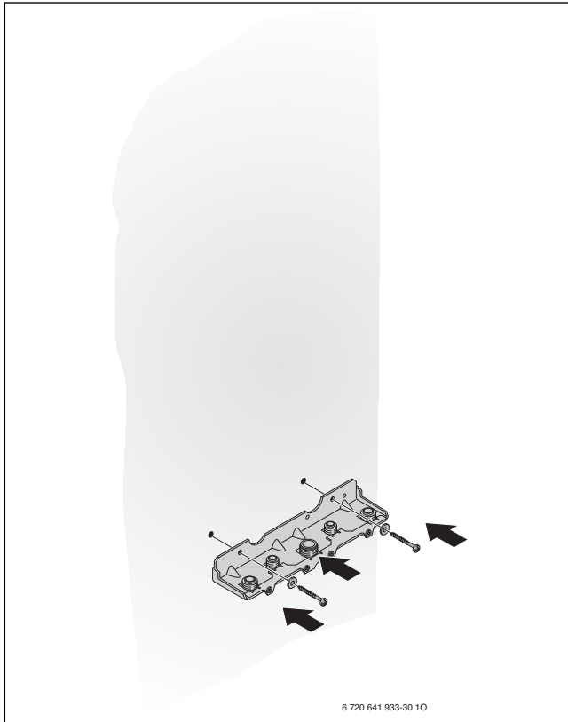
Fig. 12 Installing the hydraulics connection plate
