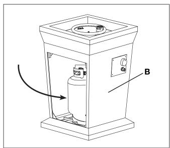
3. Turn the cylinder valve on the tank clockwise to close the propane tank. Attach the preassembled regulator from the body (B) to the cylinder valve by turning the regulator coupling nut clockwise. Make sure it is fastened securely and tighten connections by hand only.
