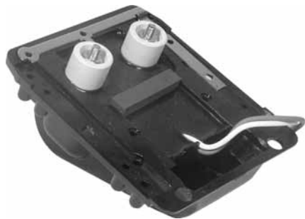
Electronic Oil Ignitor - 120 Volt Primary 50/60 Hz, 17,500 Volt Secondary, 45mA
