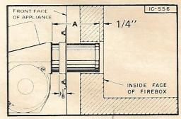
The Air Tube Length (Dimension A) is the distance from the front of the burner housing to the drain hole in the burner head. (NOTE: Adjustable flange width -1.1/8'')
