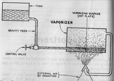
F10. 1—Elementary gravity feed induction non-mixing under flame vaporizing burner. The heat from the flame vaporizes the liquid fuel in the retort. The vapor issuing from the nozzle mixes with the air externally by induction.
