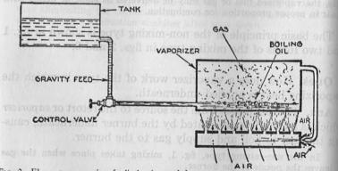
FIG. 2-Elementary gravity feedinduction mixing under flame vaporizing burner. In this type the vapor issuing from the nozzle draws in air into a mixing chamber where the vapor and air mix, the combustible mixture thus formed passes out through numerous small openings and ignites at the top.
