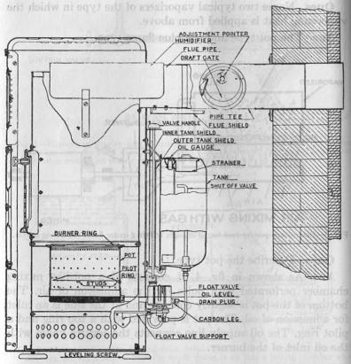
FIG. 4—Typical pot burner installation illustrating also low chimney connection and gravity oil feed with float valve. Note no manual damper is used.
