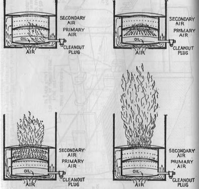
FIGS. 6 to 9—Pot burner operation. Fig. 6, starting. During this period the flame is entirely in the lower part of the pot below the pilot ring. To start, throw a lighted match or paper into the pot. Fig. 7, as the pot heats up the flame burns partly at the top of the pot and partly above the pilot ring. Fig. 8, appearance of flame when burning on a pilot fire, burning just above the pilot ring and entirely within the pot. Fig. 9, flame turned on high burning above the pot.
