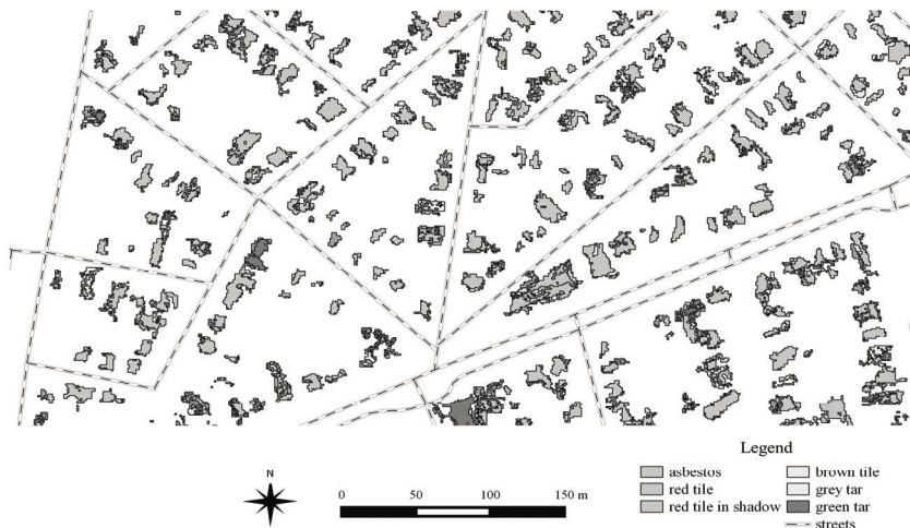
Fig. 3. Roofing types in the test area based on the SVM classification (using MNF-transformed data)
