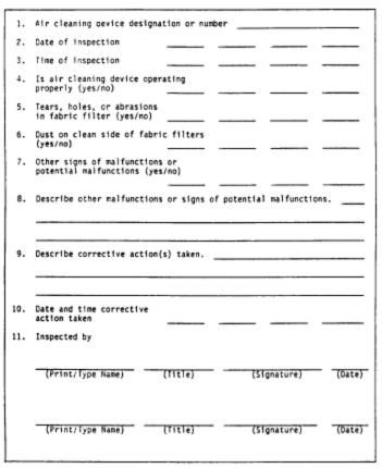
Figure 2. Air Cleaning Device Inspection Checklist
