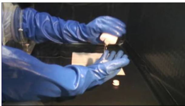
Figure 1 Pouring of powder into hands in glovebox.
