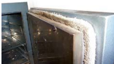
Figure 26 Asbestos rope seal on drying oven
