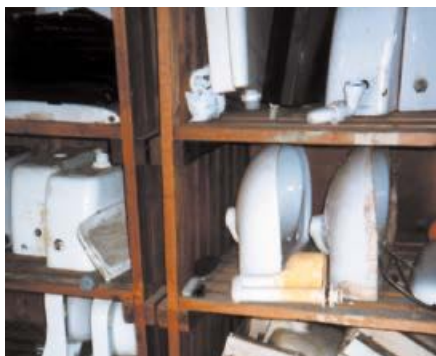
Figure 40 Asbestos-reinforced toilet cistern
