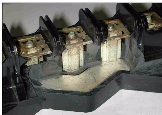
FIGURE 4 - CONDUCTING PATH FROM BUSSBAR TO STAB SOCKET
