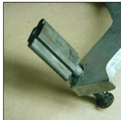
FIGURE 4 - CONDUCTING PATH FROM BUSSBAR TO STAB SOCKET
