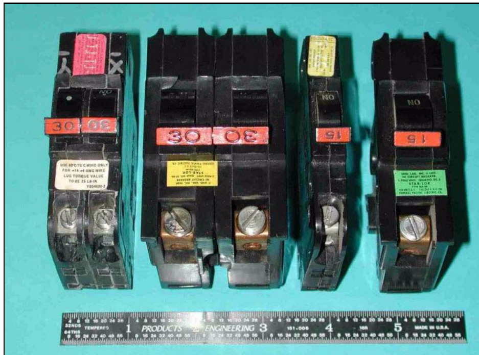
FIGURE 1 - REPRESENTATIVE SAMPLES OF HALF- AND FULL-WIDTH FPE STAB-LOK ® CIRCUIT BREAKERS (left to right: 1/2-width double pole, full-width double pole, 1/2-width single-pole, full width single-pole)
