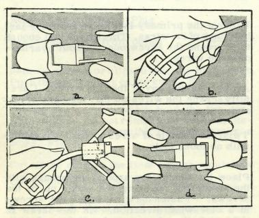
Remove the cover of the plug. Insert the wire so that the ends of the wires are enclosed in the plug. Adjust the cord. The contact is made through the insulation. Adjust the cover.
