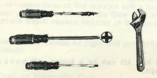
A screw holder on the shank is a great help. A screw driver with a magnetized tip which holds the screw is another convenience.
