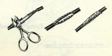
For a cord frayed or worn in the middle, cut the edges clean.
