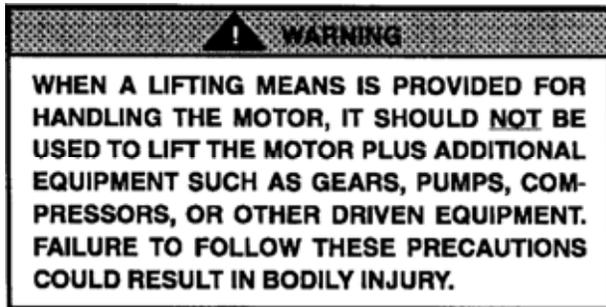
In the case of assemblies on a common base, any lifting means provided on the motor or generator should not be used to lift the assembly and base but, rather, the assembly should be lifted by a sling around the base or by other lifting means provided on the base. In all cases care should be taken to assure lifting in the direction intended in the design of the lifting means. Likewise, precautions should be taken to prevent hazardous overloads due to deceleration, acceleration or shock forces.
