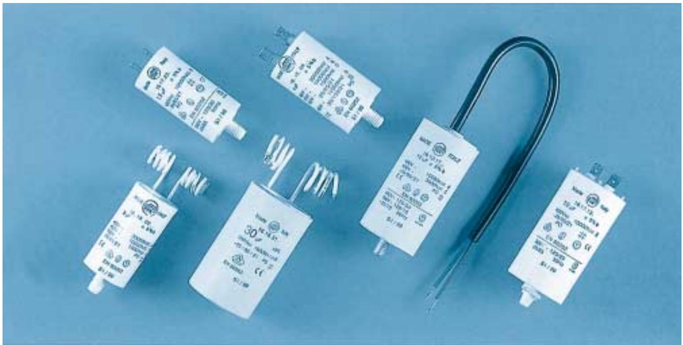
The dielectric is polypropylene film, the electrodes consist of an extremely thin metal coating obtained by vacuum evaporation. Case and cover are made with self-extinguishing plastic material, the capacitive element is sealed with polyurethanic resin.
