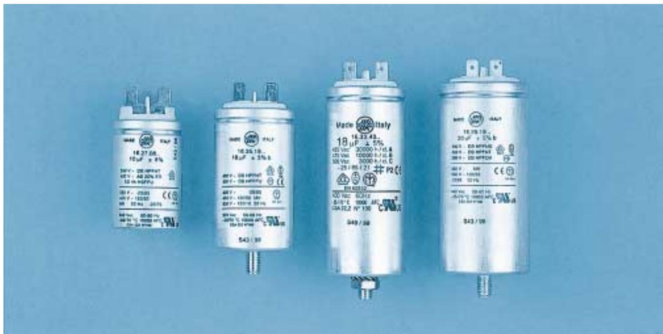
The dielectric is polypropylene film, the electrodes consist of an extremely thin metal coating obtained by vacuum evaporation.
