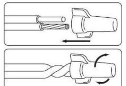
Use only on Copper to Copper (Cu/Cu) wire combinations. For use in dry locations only. Temperature rating: 105 C (221 F) maximum. 600 volts maximum building wire; 1000 volts signs or lighting fixtures. UL 486C Listed and CSA C22.2 #188 Certified Complies with Federal Specification W-S-61D
