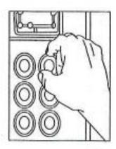
Next, plug in and turn ON the lamp or radio at the receptacles other outlet to make sure the power is OFF at both outlets. If the power is not OFF, stop work and call an electrician to complete the installation.
