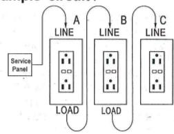
Placing the GFCI in position A will also provide protection to load side receptacles B and C. On the other hand, placing the GFCI in position C will not provide protection to receptacles A or B. Remember that receptacles A, b, and C can be in different rooms.
