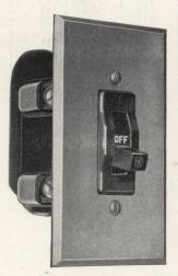
**FUNCTION:** These Circuit Breakers serve both as master control switches, governing groups of lighting or convenience outlets (occasionally both), and as means of overload and short-circuit protection. These breakers eliminate fuse replacements, and the practice of hazardous over-fusing and provide accessible localized control at convenient decentralized points for re-establishing circuits opened by overloads or other abnormal conditions.
