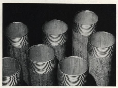
G-E White Rigid Conduit is made of rimmed steel—hot-dipped galvanized and Glyptal coated inside and out. Avoids split seams, bends easily, and threads easily
