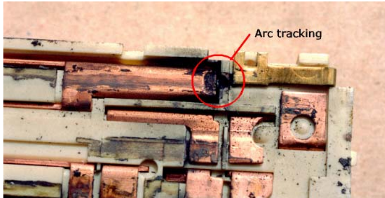
Fig. 7. Arc tracking failure of an automotive ignition switch, in nominal 12 VDC service (Photo: Chris Bloom).
