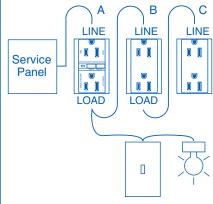
Always place Outlet Branch Circuit Type AFCI in position A. All outlets of the protected branch, including lighting and receptacle outlets, must be connected to the load side of the AFCI.
