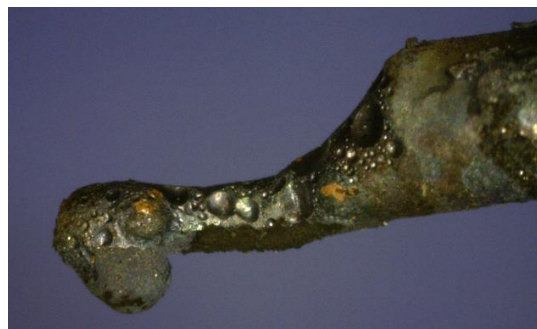
Figure 4-22. Pitting of copper wire due to fire-melting (LEV391).
