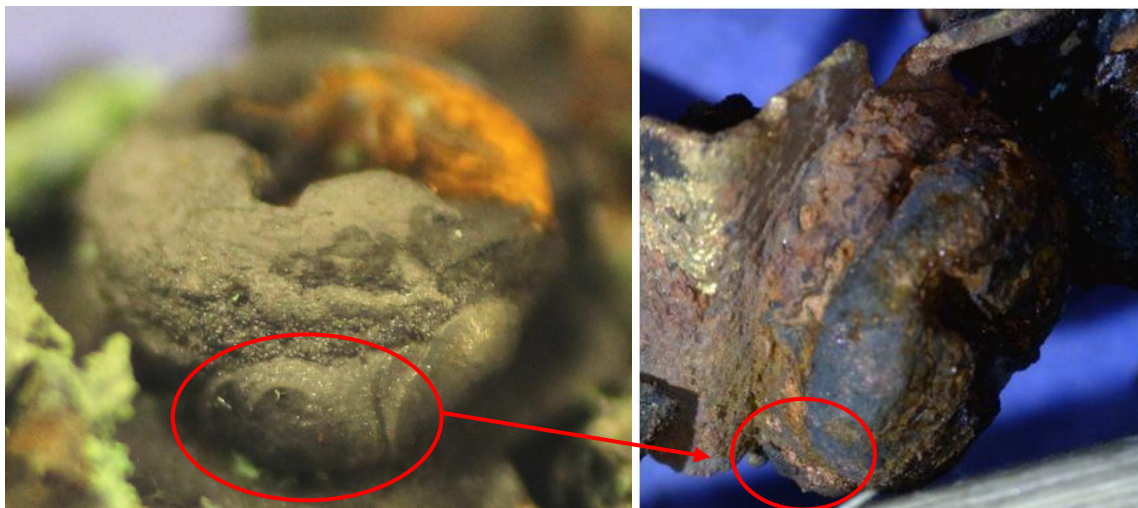
Figure 3-79. Welded conductor with curved striations before (left) and after (right) furnace fire exposure (PSE021).
