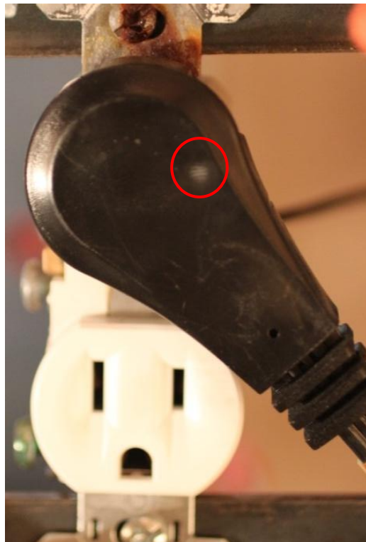
Figure 2-13. Overheating and discoloration of black plug with plated blade (PSE285; 0.01 kg).
