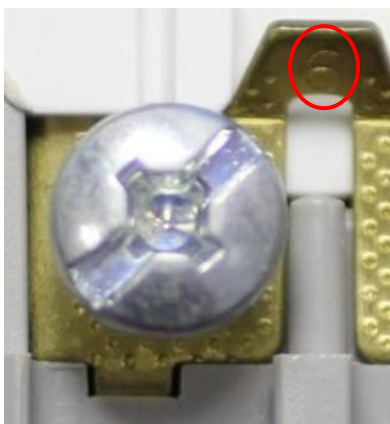
Figure 4-11. Typical stamped number (circled), bent brass plug contact with crisp edges from an exemplar PVC receptacle.
