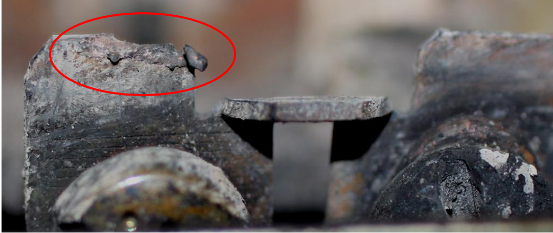
Figure 4-5. Notch in brass plug contact which is not round and smooth (LEV144).
