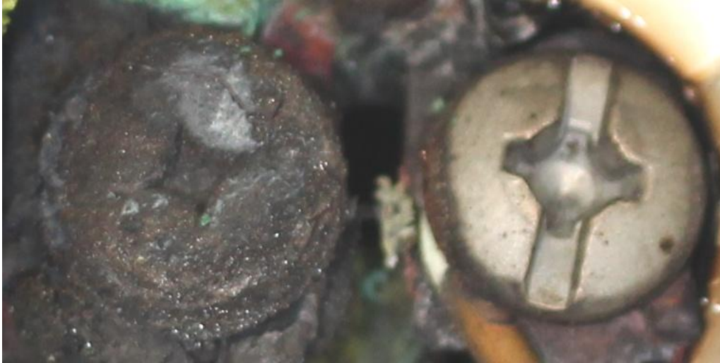
Figure 2-62. Enlarged screw head from receptacle PSE129.
