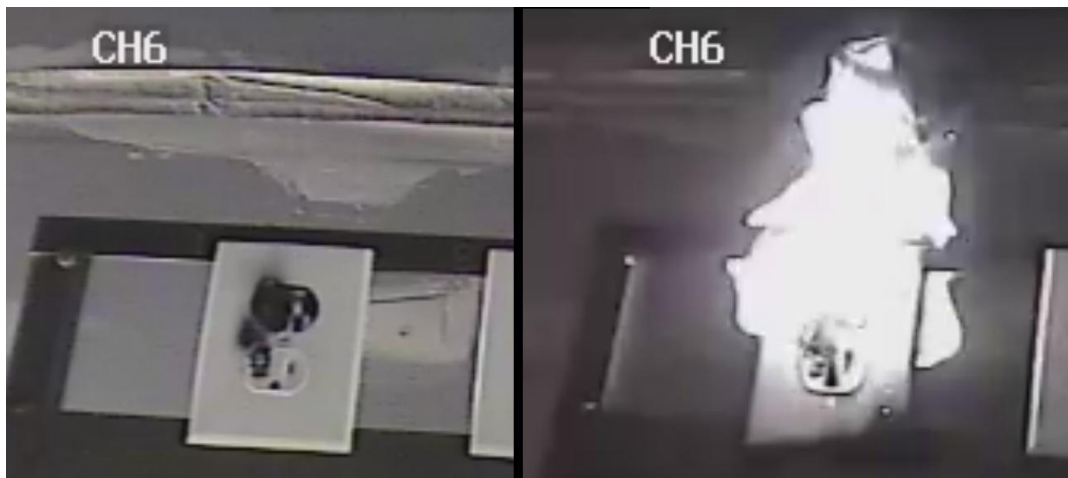
Figure 2-46. Flaming ignition of receptacle in box (before ignition (left) and 21 seconds after ignition (right)).
