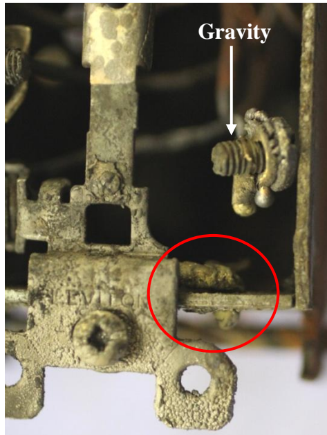
Figure 3-38. Photograph of melted brass receptacle contact showing round globules, effects of gravity and dripping brass (LEV363, non-energized).
