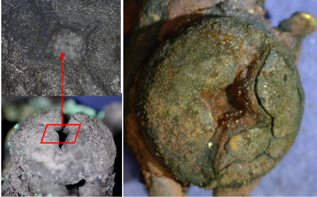
Figure 3-81. Enlarged screw head from PVC receptacle before (left) and after (right) the furnace exposure (PSE132).
