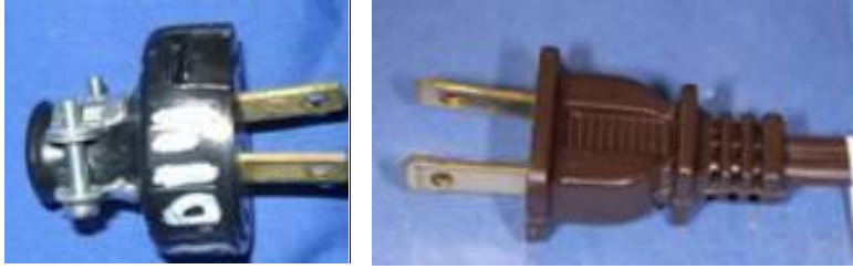
Figure 1-5. Solid brass (left), folded brass (right) plug blades.
