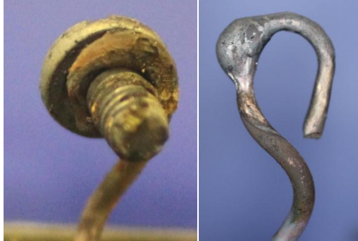
Figure 3-42. Tapering of melted copper wiring on a polypropylene receptacle (energized, LEV365, left) and a thermoset receptacle (non-energized, C023, right).
