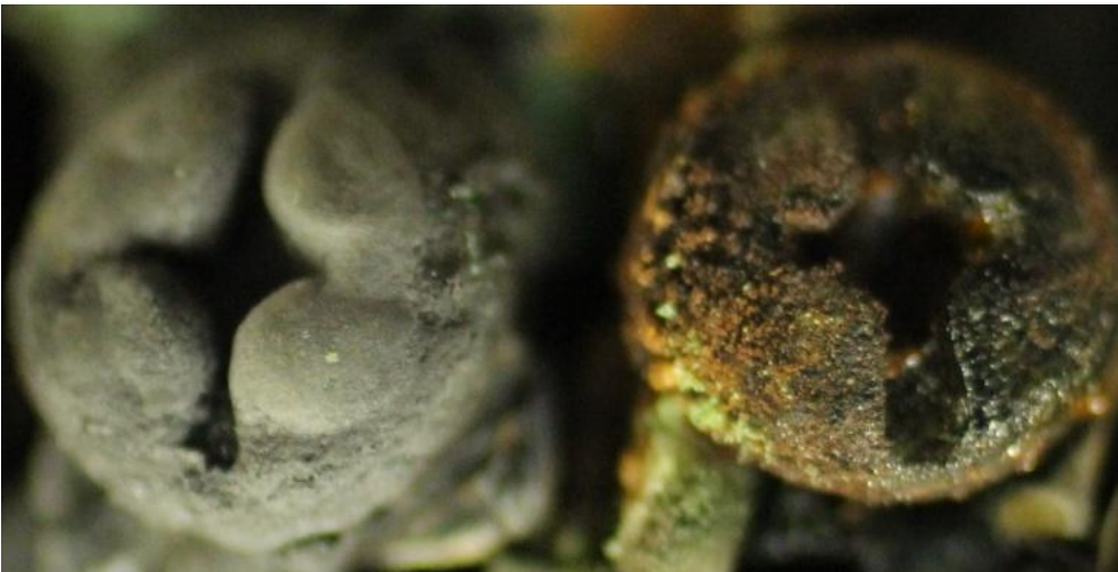
Figure 2-63. Enlarged screw head from receptacle PSE170.
