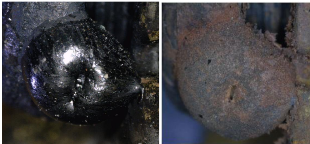
Figure 3-98. Severed conductor end on screw side from polypropylene (LEV272) receptacle before (left) and after (right) furnace exposure.
