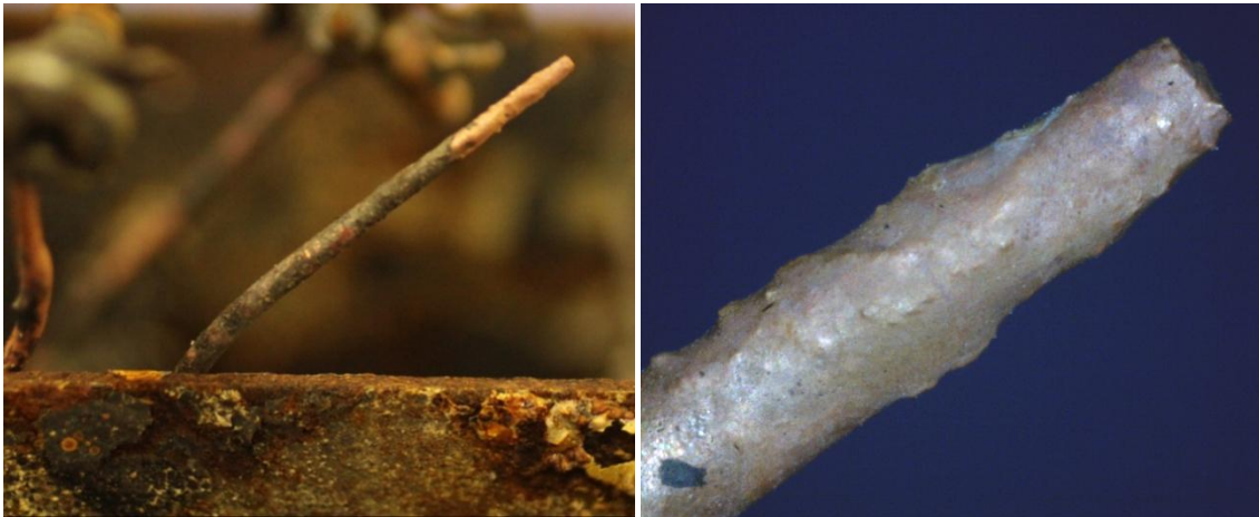
Figure 3-43. Photographs of melted copper wiring from a PVC receptacle showing tapered shape, irregular surface, and flat end (energized, PSE369).
