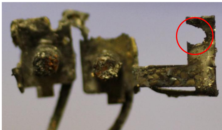
Figure 4-24. Holes formed on brass plug contacts due to fire-melting (PSE381).
