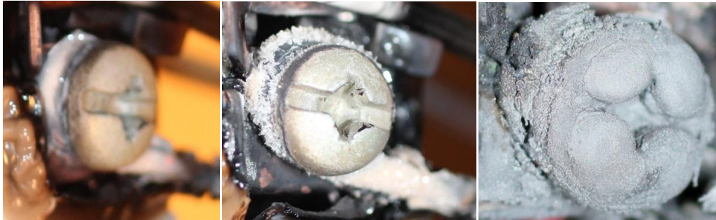
Figure 2-44. Development of enlarged screw head on receptacle PSE170 at T = 0 hours (left), T = 21.6 hours (center) and T = 29.2 hours (right).
