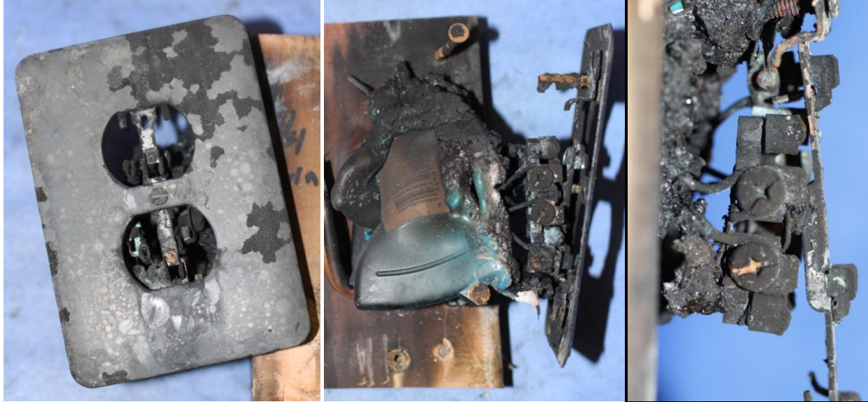
Figure 3-31. Photographs of steel faceplate (left), PVC outlet box (center) and poly propylene receptacle (LEV160, right).
