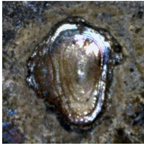
Figure 4-6. Notch in steel faceplate which is round and smooth (PSE331).
