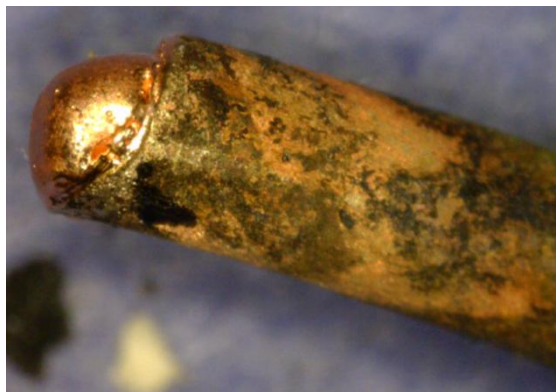
Figure 4-7. Round and smooth bead on end of wire severed by arcing (E001).
