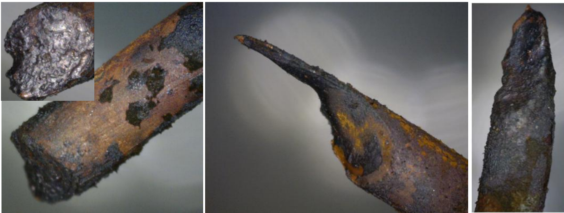
Figure 3-44. Photographs of three melted copper wire ends from a single non-energized polypropylene receptacle (LEV371): flat (left with blowup of flat face), pointed (center), and tapered (right).
