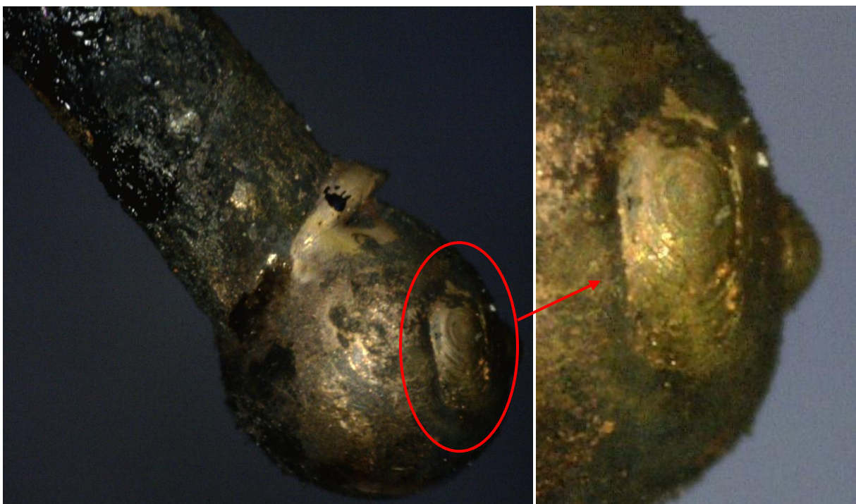
Figure 4-10. Arcing damage on copper wire showing resolidification waves (LEV172).
