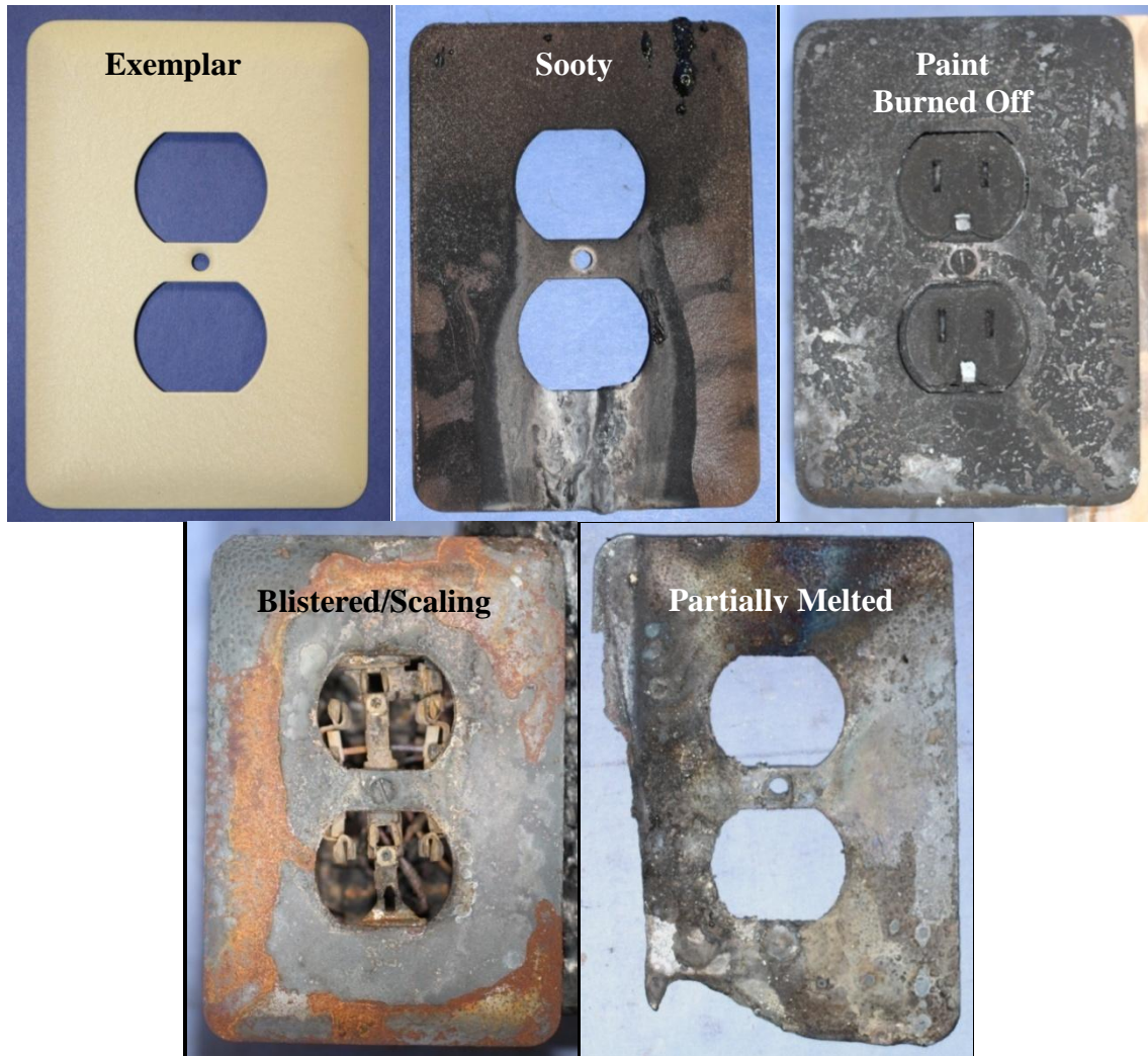
Figure 3-24. Photographs of damage progression in steel faceplates.
