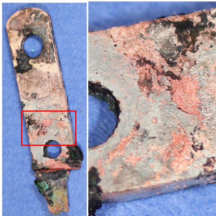
Figure 2-28. Loss of plating and dezincification of low profile plug blade; nominal retention force of 0.01 kg (LEV286).
