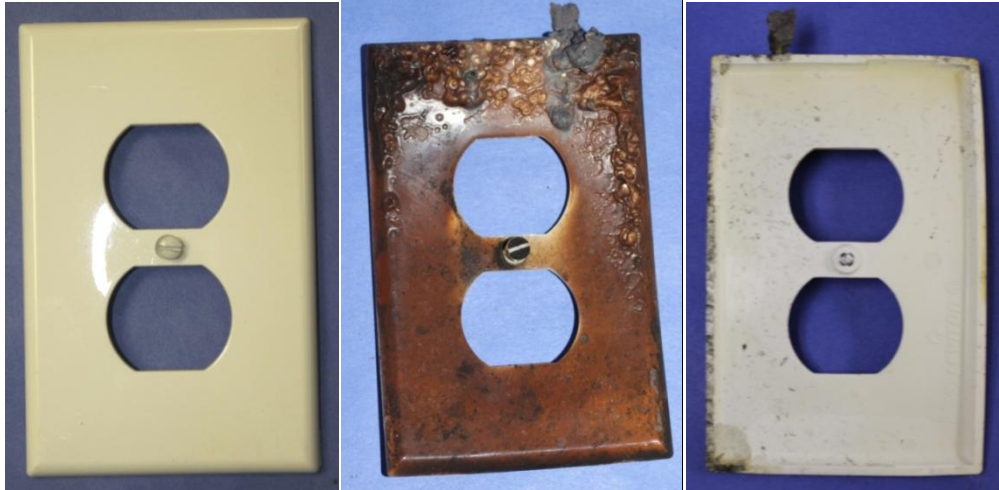
Figure 3-21. Photographs of damage progression in nylon faceplates, exemplar (left) and blistered/partially melted front (center) and back (right).
