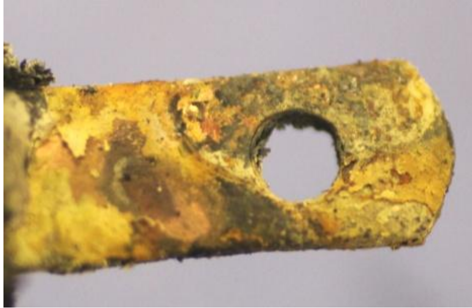
Figure 2-79. Loss of plating and dezincification on hot plug blade (LEV060).
