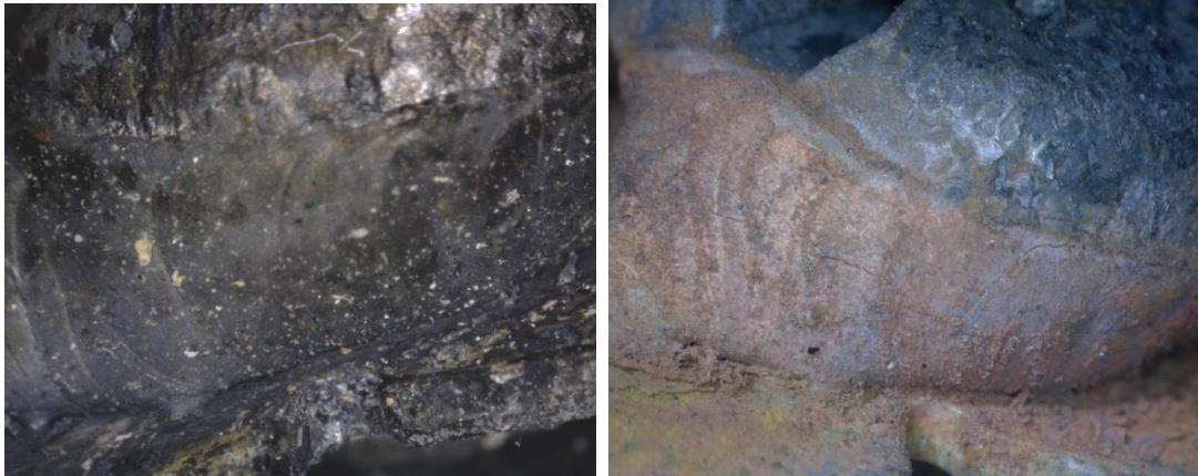
Figure 3-77. Welded conductor with curved striations before (left) and after (right) furnace fire exposure (LEV272)
