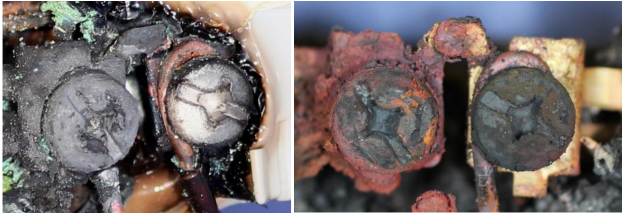
Figure 3-80. Enlarged screw head from PVC receptacle before (left) and after (right) furnace exposure (PSE023).
