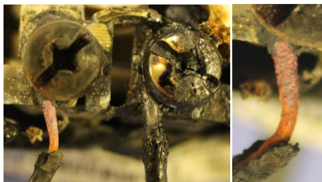
Figure 2-18. Thinned and pitted wire from oxidation (LEV009).
