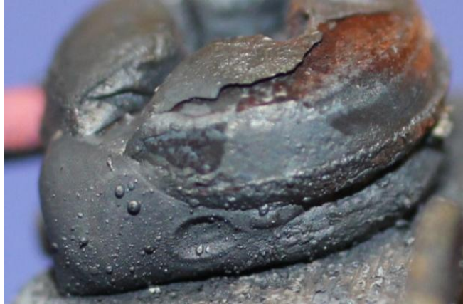
Figure 2-59. Partially welded conductor; no curved striations (LEV127).
