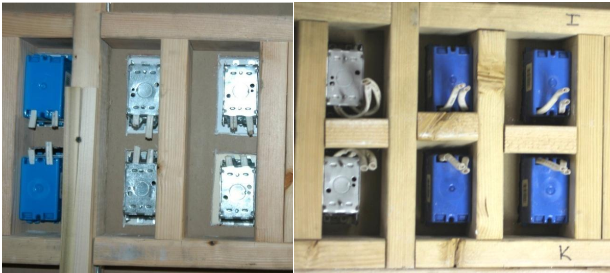
Figure 3-2. Typical outlet box installation for Test 1 (left) and Tests 2 through 8 (right).
