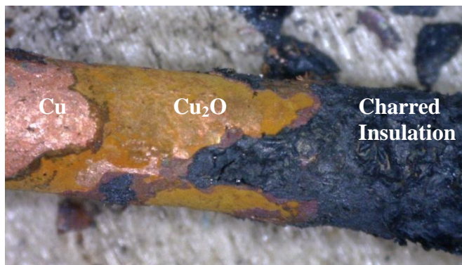
Figure 2-15. Oxidation of wire, showing layer of Cu 2 O in center and underlying copper (PSE170).
