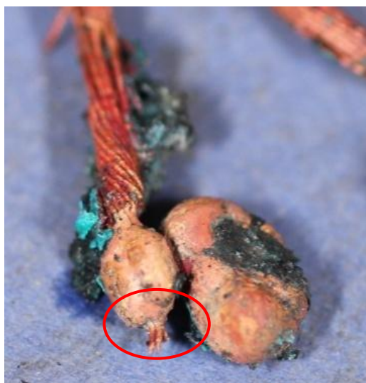
Figure 3-50. Photograph of melted stranded copper wiring for an energized extension cord from a thermoset receptacle; wire strands running through melt globule circled in red (E098).
