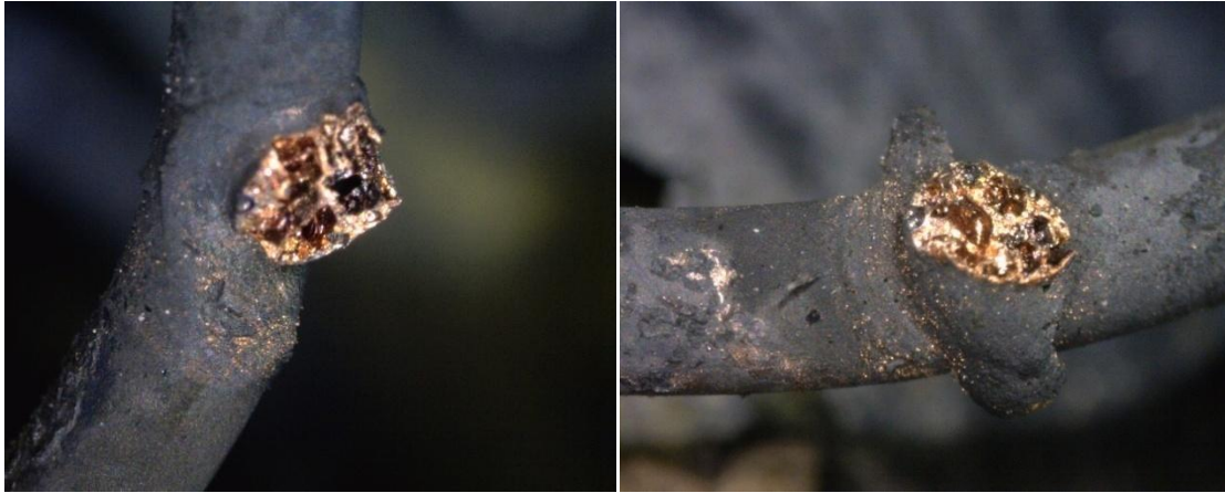
Figure 3-70. Photograph of arcing in receptacle hot and neutral wires showing internal porosity from a thermoset receptacle (B020).
