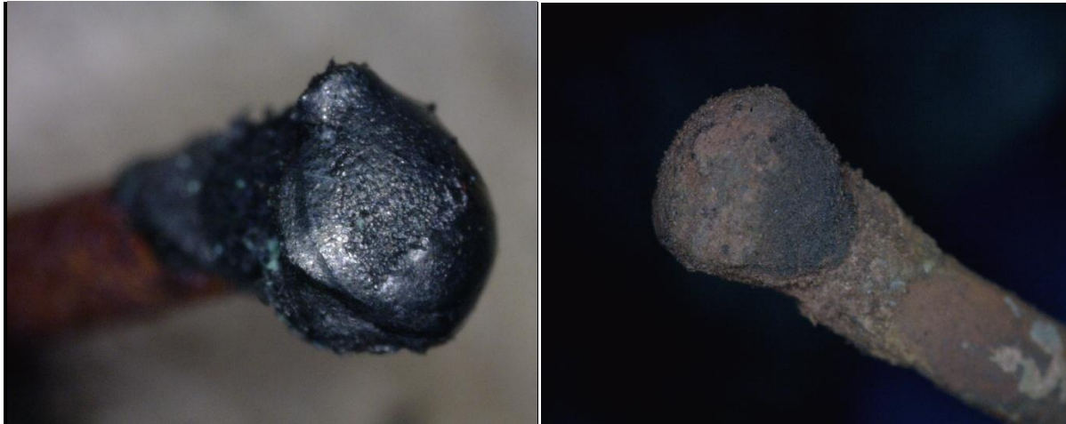
Figure 3-97. Photographs of severed conductor end on wire from PVC (PSE023) receptacle before (left) and after (right) furnace exposure.
