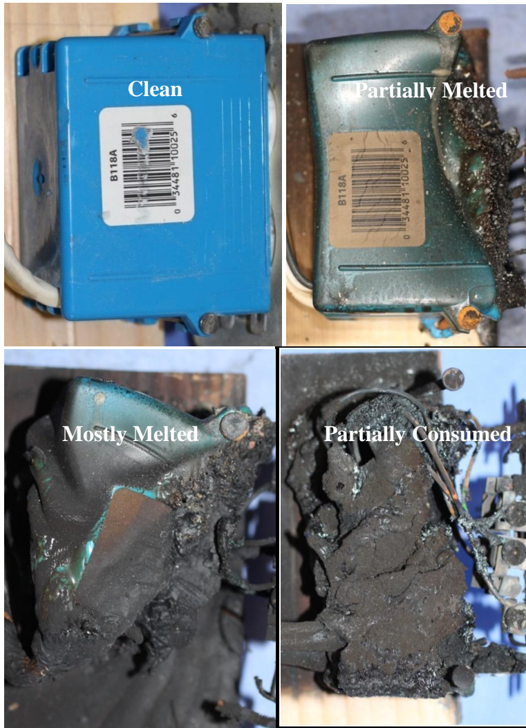
Figure 3-26. Photographs of damage progression in PVC outlet boxes (increasing thermal insult from top left to bottom right).
