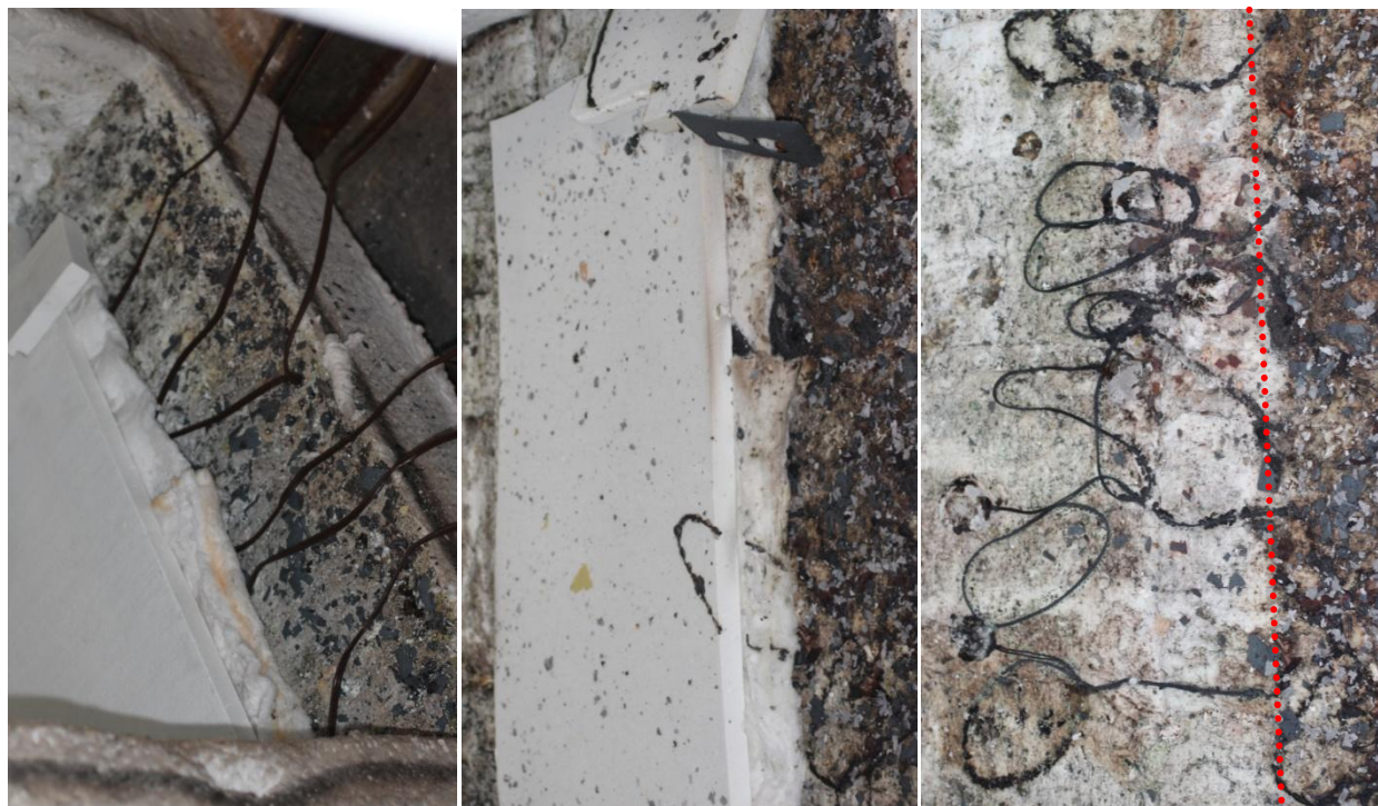
Figure 3-40. Extension cord wiring covered with insulation prior to test (left), with insulation after test (center) and with insulation removed (right) after furnace Test 4.
