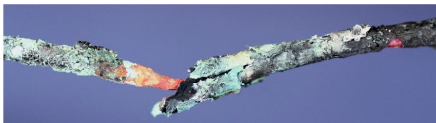
Figure 2-19. Thinned and pitted wire from oxidation (PSE263).
