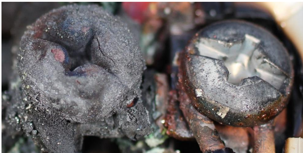
Figure 2-61. Enlarged screw head on receptacle PSE134.
