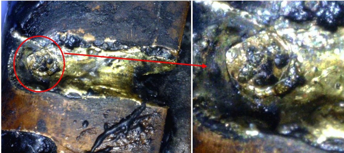
Figure 4-13. Arcing damage on brass plug contact showing large voids (LEV266).
