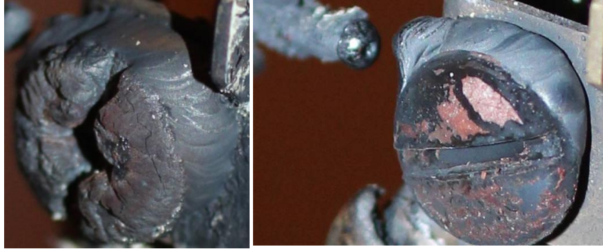
Figure 2-41. Curved striations from glow movement on receptacles, receptacle LEV275 (left) and E003 (right).
