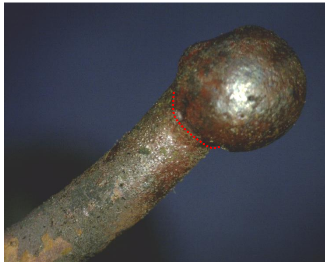
Figure 3-41. Melted copper wiring from a non-energized polypropylene receptacle showing line of demarcation (LEV389).
