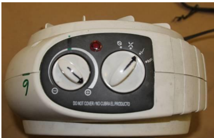
Figure 3-9. Heater setting for compartment fire tests.
