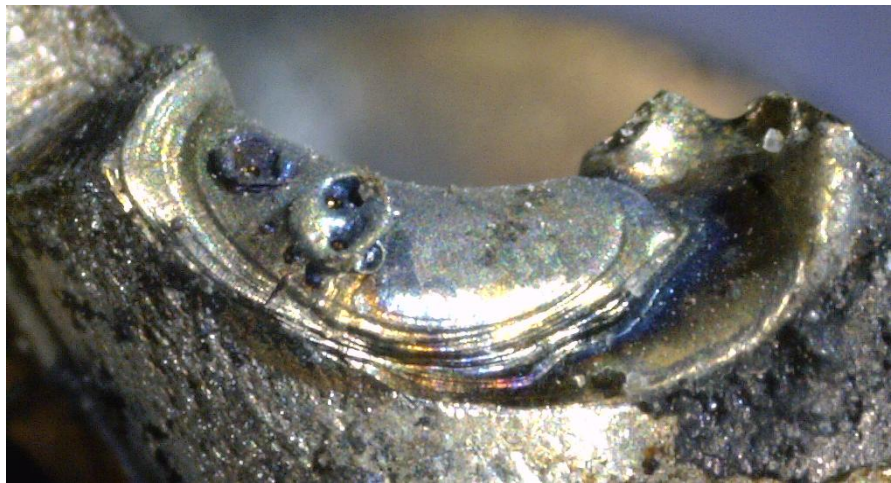
Figure 4-9. Arcing damage on grounding strap showing resolidification waves that are more pronounced on the major axis (LEV174).
