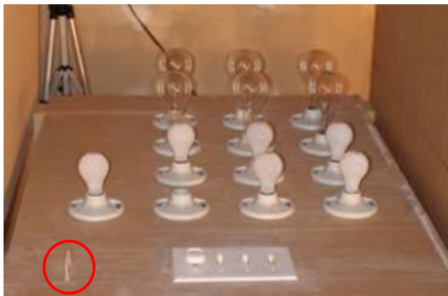
Figure 2-6. Photograph of light bulb load bank. Note: neutral wire circled.
