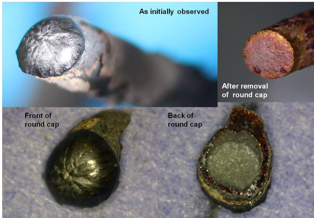
Figure 2-70. Round, shiny severed conductor end showing round cap and flat underneath (LEV173).
