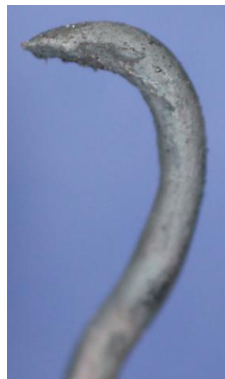
Figure 4-21. Gradual necking of copper wire due to fire-melting (C023).
