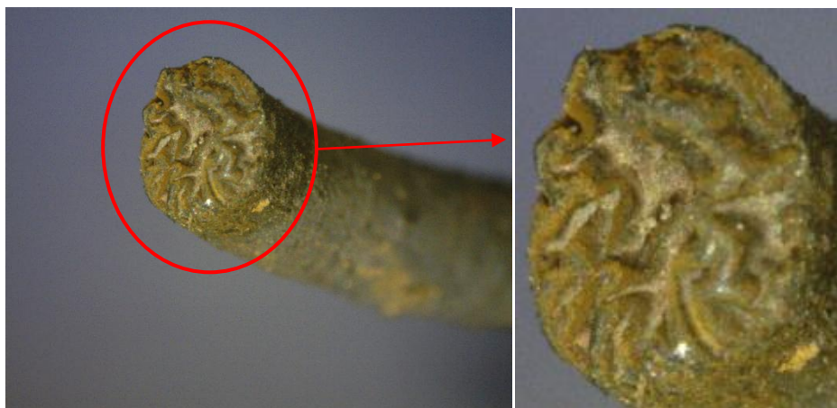
Figure 3-45. Photograph of melted copper wiring showing a flat end with pitting from a non-energized PVC receptacle (PSE384).
