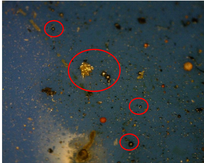
Figure 4-15. Spatter from arcing, deposited on PVC outlet box (LEV172).
