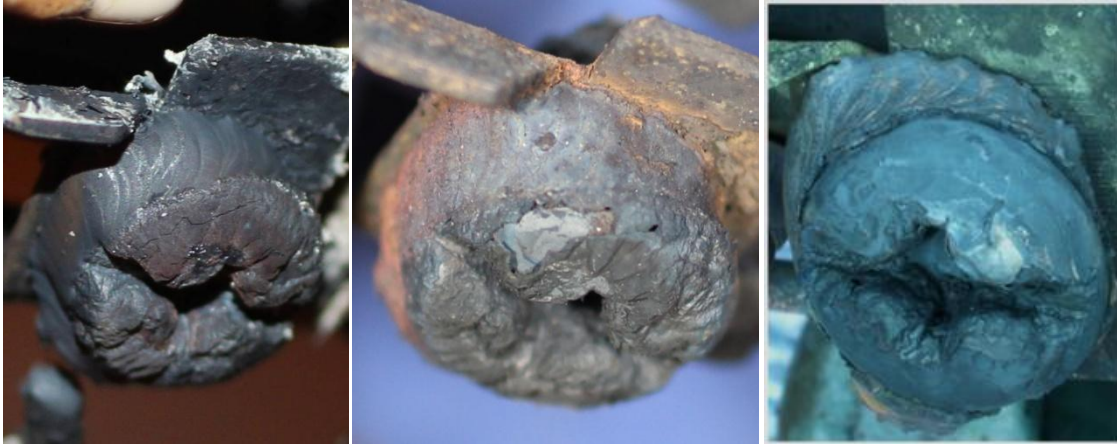
Figure 3-78. Welded conductor with curved striations before furnace exposure (left), after furnace exposure (center), and after furnace exposure with ultrasonic cleaning (right), (LEV275).
