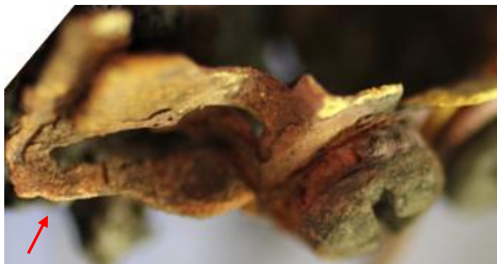
Figure 3-99. Photograph of internal plug contacts thinned by oxidation and overheating from PVC receptacle (PSE023).
