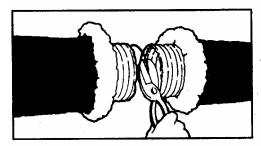
Slide at least 1" [25 mm] of core over fitting and past the bead. Seal core to collar with at least 2 wraps of duct tape. Secure connection with clamp placed over the core and tape and past the bead.
