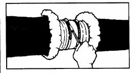
Pull jacket and insulation back over cores. Tape jackets together with at least 2 wraps of duct tape.
