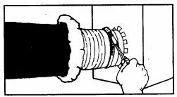
Pull jacket and insulation back over core. Tape jacket with at least 2 wraps of duct tape. A clamp may be used in place of or in combination with the duct tape.
