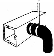
5. Vertically installed duct should be stabilized by support straps at a maximum of 6 feet (1829 mm) on center.
