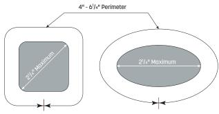
For Residential Applications, the ICC permits the use of larger handrail sections that meet the Type II Definition as noted to the right. This applies to handrail sections with a perimeter greater than 6 3/4"
