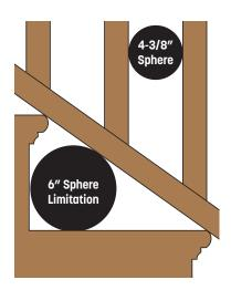
4" sphere rule - no opening large enough to pass a 4" sphere is permitted.
