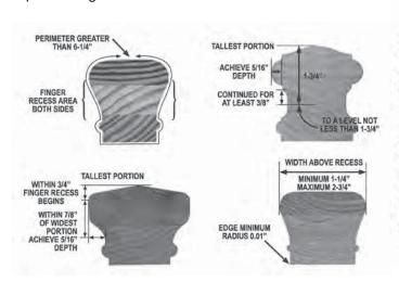
Equivalent Graspability is defined as: Handrail gripping surfaces with a non-circular cross section shall have a perimeter dimension of 4 inches (100 mm) minimum and 6" maximum, and a cross section dimension of 2 1/4" (57mm) maximum.
