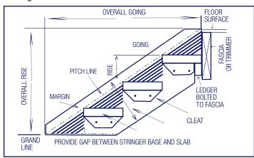
**CALCULATE CLEAR TREAD WIDTH** Width the acceptable riserheight calculated as in step 2 above, now calculate the preferred clear step width. (Note that the MINIMUM acceptable clear tread width will be 240 mm.)
