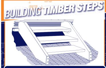
There is often a need for steps as an access to a deck or for use between stairways can be much the same as open detailing which avoids trapped moisture or exposed end grain of the members should be used. A basic open stairway consists of the two stair stringers and the treads. The supporting members of a stair are these stringers which are used in pairs spaced at up to about I metre apart. The overall height of steps from ground line to deck or landing should not exceed 1 metre.
