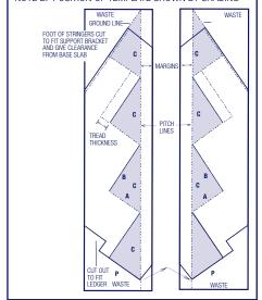
similar fastenings inserted in the existing patio floor or path. If new concrete slab is required this should be level and sufficiently wide, at least, to form another standard size ground level tread and located to conform to the step/tread pattern. **Example** Tread length 900 mm Minimum concrete slab 1200 x 300 x 100 mm Distance between centres of brackets and stringers 945 mm.
