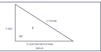
CALCULATE STRINGER LENGTH Measure C the pitch length on your template. Multiply pitch length by the number of risers to give overall length of pitch line.
