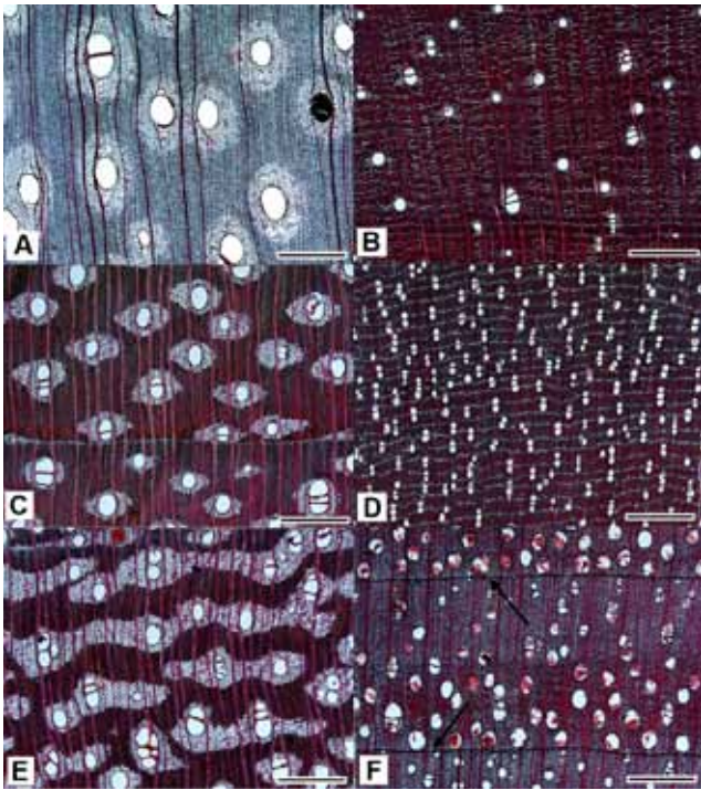
Figure 3–11. Transverse sections of various woods showing a range of hardwood axial parenchyma patterns. A, C, and E are woods with paratracheal types of parenchyma. A, vascentric parenchyma in Enterolobium maximum ; note that two vessels in the middle of the view are connected by parenchyma, which is the feature also shown in E; the other vessels in the image present vascentric parenchyma only. C, aliform parenchyma in Afzelia africana ; the parenchyma cells are the light-colored, thin-walled cells, and are easily visible. E, confluent parenchyma in Afzelia cuazensis . B, D, and F are woods with apotracheal types of parenchyma. B, diffuse-in-aggregate parenchyma in Dalbergia stevensonii . D, banded parenchyma in Micropholis guyanensis . F, marginal parenchyma in Juglans nigra ; in this case, the parenchyma cells are darker in color, and they delimit the growth rings (arrows). Scale bars = 780\ \mu\text{m} .
