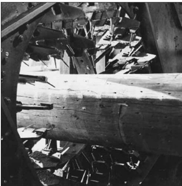
Figure 15-4. Deep incising permits better penetration of preservative.
