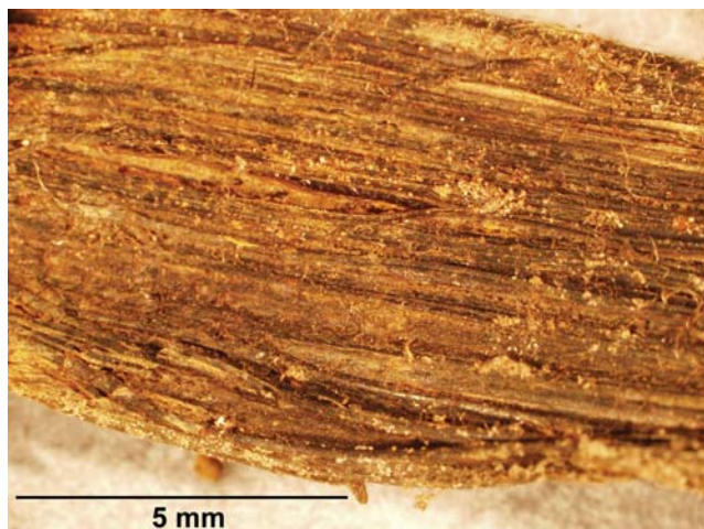
Figure 2. Close-up view of the "textured" side of the cording. Note that individual fibers can be seen running parallel to the length of the cording proper.
