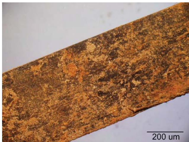
Figure 3. Close-up view of the "smooth" side of the cording. Note that while slight longitudinal striations are evident, no individual fibers are distinguishable.
