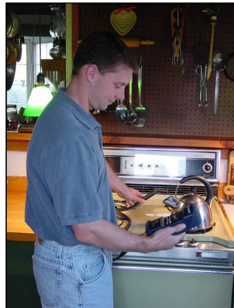
Testing gas oven for CO emission level
