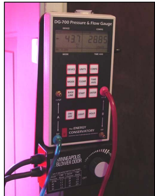
DG-700 digital manometer from The Energy Conservatory
