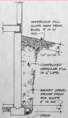
For a dry basement, keep water away from the foundation walls. Good surface drainage and proper footing drains are the first priorities.
