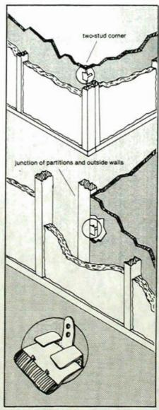
The two-stud corner (top) provides adequate structual support, saves wood, and allows easy and full insulation at building corners. Using drywall clips or a partial 1x3 backer allows one edge of drywall to float at the building corner, minimizing cracks here. A similar detail (above) will work at the junction of partitions and outside walls.
